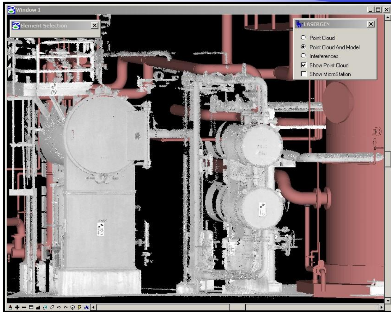
Laser Scan Point Cloud Overlay within 3D CAD Environment
